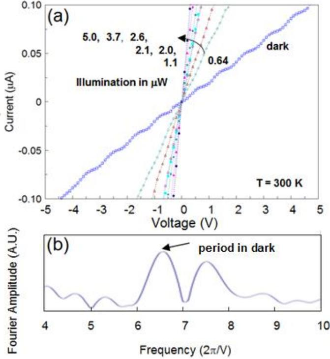
**Figure 2.** (a)  $I_d$  as a function of  $V_d$  with light power as a parameter. (b) Fourier transform of  $I_d(V_d) - cV_d$ , where  $c$  is a constant. The peak is at  $2\pi/V = 6.6 \text{ V}^{-1}$ , corresponding to the staircase period of  $\Delta V = 0.95 \text{ V}$ .
