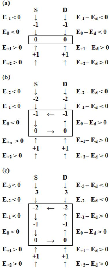
**Figure 4.** Evolution in the number of electrons on the island for different bias  $V_d$ . (a) region A of zero current, with the number of thermodynamically allowed island electrons ( $N$ ) is 0, (b) region B of unit current with  $N = -1$  and 0, and (c) region C of two units of current with  $N = -2, -1$ , and 0. Arrows indicate how tunneling occurs and  $N$  changes.
