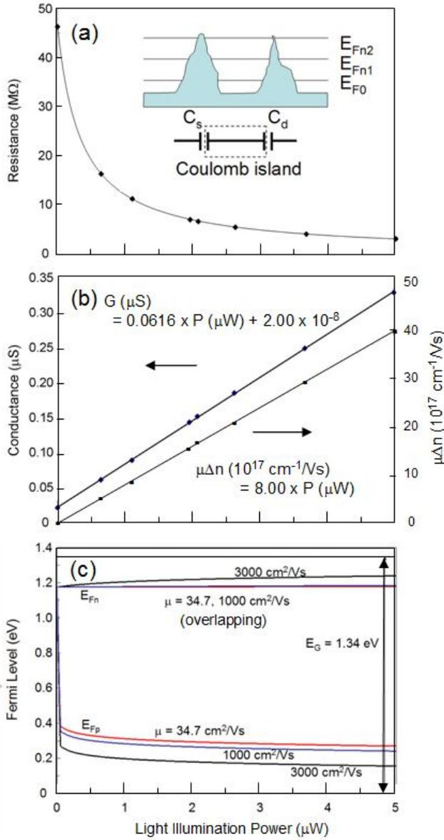
**Figure 5.** (a) Resistance  $R_{\text{tot}}$  as a function of light illumination power  $P$ , where each dot represents a measured point. Inset: Schematic energy band diagrams for a Coulomb island and barriers for Fermi levels  $E_{F0}$ ,  $E_{F1}$ , and  $E_{F2}$ . (b) Conductance  $G$  and  $\mu\Delta n$  as a function of  $P$ . (c)  $E_{Fn}$  and  $E_{Fp}$  as a function of  $P$  for representative electron mobility  $\mu$  values, 34.7 [17], 1000, and 3000 cm<sup>2</sup>/Vs.
