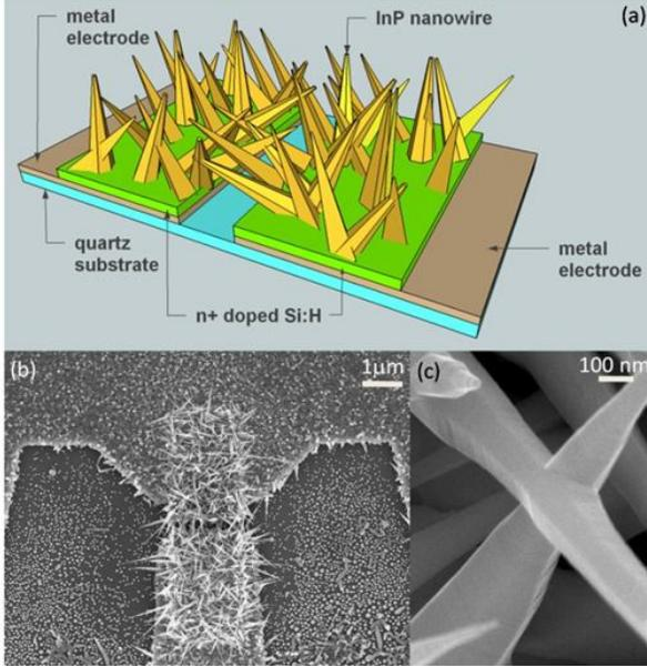
**Figure 1.** (a) Schematic of a fabricated InP nanowire (NW) photoconductor. (b) Scanning electron microscope (SEM) image (top view) of a representative InP NW photoconductor. InP NWs were selectively grown on the pair of  $n^+$ -doped Si:H electrodes. (c) SEM image of a point where two nanowires were fused.
