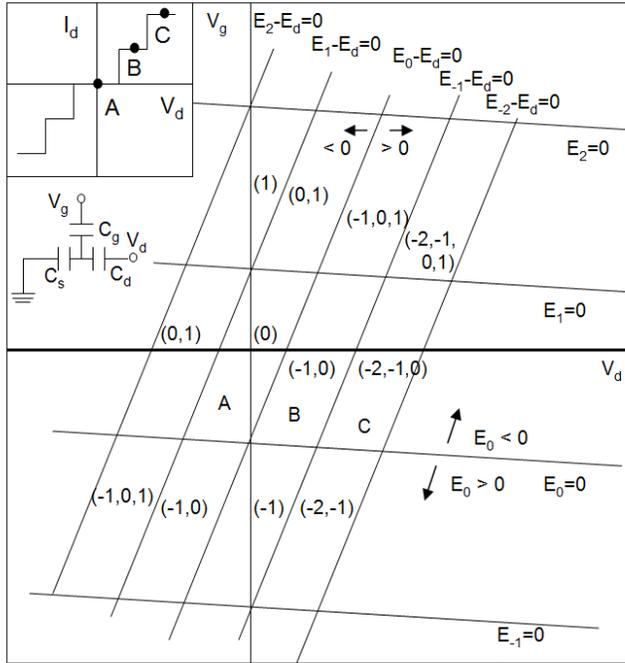
**Figure 3.** Internal energy change  $\Delta(N,k) = E_N - E_k$  after incoming electron tunneling to the island from electrode k in the  $V_g$ - $V_d$  plane. If  $E_N - E_k < 0$ , an electron tunnels *in* from electrode k to the island with  $N$  *final* electrons (the island electrons change from  $N-1$  to  $N$ ). If  $E_N - E_k > 0$ , an electron tunnels *out* from the island with  $N$  *initial* electrons to electrode k (the island electrons change from  $N$  to  $N-1$ ).
