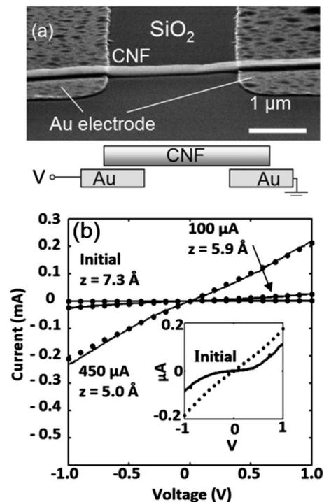
FIG. 1. (a) SEM image of a Au-CNF-Au system on SiO<sub>2</sub> substrate. (b) Measured  $I$ - $V$  before and after multiple current stressing. Current stressing conditions are shown with current magnitude and duration time. Solid circles are modeling results at 300 K, with fitted  $z=7.3$ , 5.9, and 5.0 Å and measured  $S=0.125$   $\mu\text{m}^2$  from SEM.
