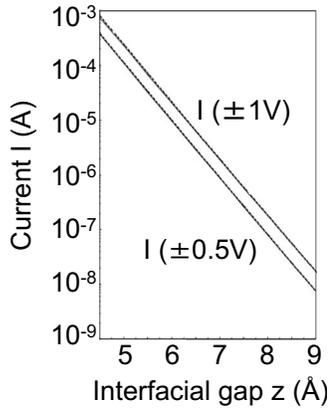
FIG. 4. Current  $I$  at  $\pm 1$  and  $\pm 0.5$  V as a function of interfacial gap  $z$  at 300 K with  $S=0.125 \mu\text{m}^2$ . Negative biases are shown with solid lines and positive biases are shown with broken lines, which virtually overlap.
