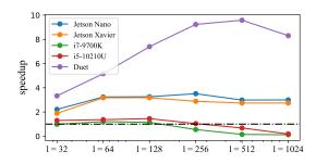
Fig. 5. Speedups of BH Gau application across different leaf node sizes on our five evaluation platforms.
