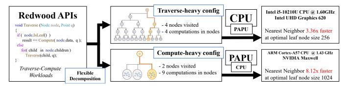
Fig. 2. The flow of Redwood: (left) User uses Redwood APIs to implement traverse-compute workloads. (middle) The workload can be easily configured to target SMHSs with different relative throughputs between CPU and PAPU. (right) Workload now can be used to evaluate different SMHSs.
