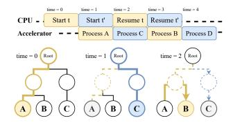
Fig. 3. Traverser execution timeline: At each time stamp, the CPU traversal trace is highlighted with a solid colored line. The leaf node that is being processed by the PAPU is shaded in grey. The dotted color lines are traversals that are suspended and will be resumed later.
