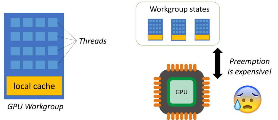
On GPUs, preemption is difficult due to the large state that needs to be saved. A GPU workgroup's state contains up to **256 threads** and a **local cache**. Efficiently saving and restoring is non-trivial.
