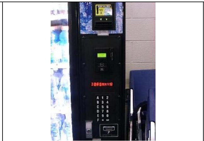
Figure 2: Illogical payment method (the slot for bills is separated from the slot for coins)
