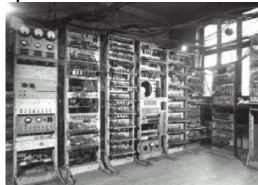
Manchester SSEM (1948) – “Baby”: Small Scale Experimental Machine. Mark 1 prototype. http://www.computer50.org/mark1/new.baby.html
