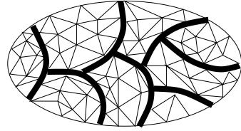
**Figure 2:** The thick black line, the fence, is a itself collection of  $o(n)$  triangles.
