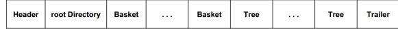
Figure 1: Physical structure of a ROOT file [8]. Baskets contain data and trees include only metadata.
