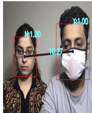
Fig.20. Status shows N and Y respectively and the distance of approximately 10.27 inches
