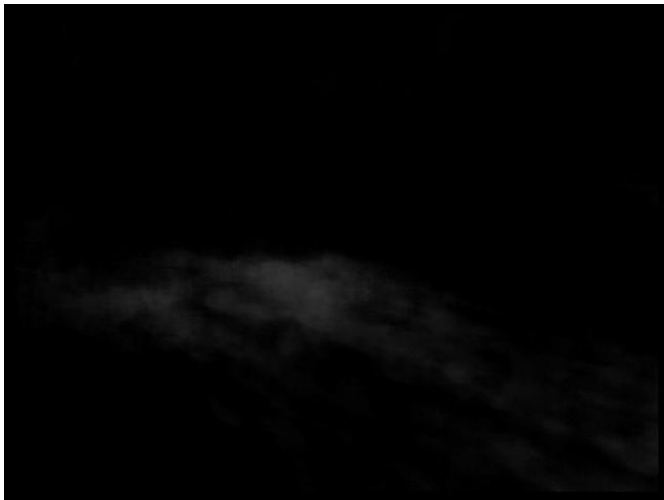
Figure 8: Contents of accumulator buffer for 90 frames. Cell counts have been normalized where black is zero and white is 1.
