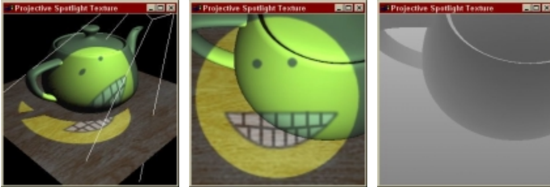
Figure 2. A shadow mapped scene rendered from the eye's point of view (left), the scene as rendered from the light's point of view (center), and the corresponding depth/shadow map (right).
