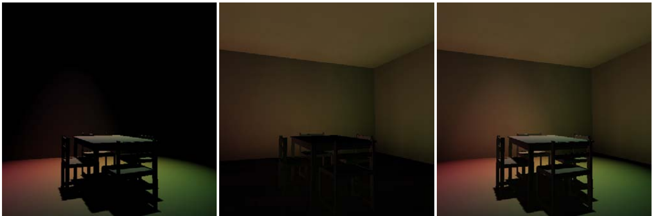
Figure 8: On the left, local illumination and shadow mapping is shown. The indirect illumination (center image) is approximated from the RSM and combined to obtain the final image (right).
