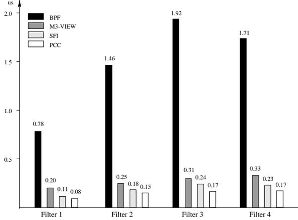
Figure 8: Comparison of average per-packet run time.
