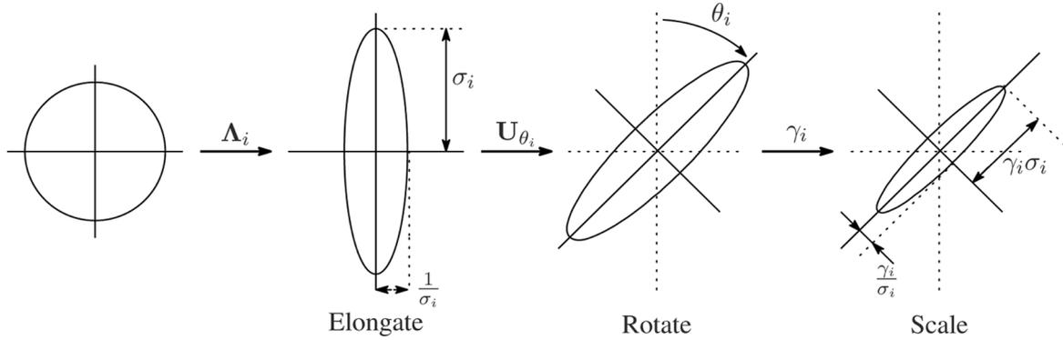
Fig. 9. Schematic representation illustrating the effects of the steering matrix and its component ( $\mathbf{C}_i = \gamma_i \mathbf{U}_{\theta_i} \mathbf{\Lambda}_i \mathbf{U}_{\theta_i}^T$ ) on the size and shape of the regression kernel.
