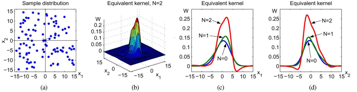
Fig. 6. Equivalent kernels for an irregularly sampled data set shown in (a); (b) is the second-order ( $N = 2$ ) equivalent kernel. The horizontal and vertical slices of the equivalent kernels of different orders ( $N = 0, 1, 2$ ) are compared in (c) and (d), respectively. In this example, the kernel  $K_{\mathbf{H}}$  in (20) was modeled as a Gaussian, with the smoothing matrix  $\mathbf{H} = \text{diag}[10, 10]$ .
