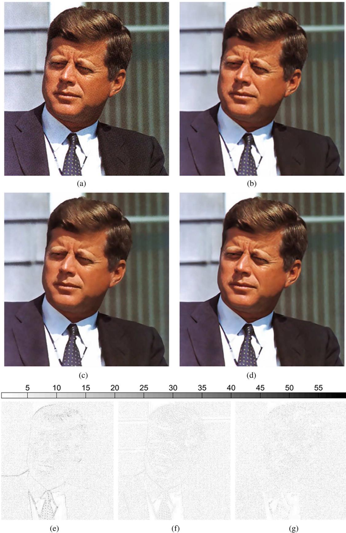
Fig. 14. Performance of different denoising methods are compared in this experiment on a color image with real noise; (e)–(g) show the residual between given noisy image and the respective estimates. (a) Real noisy image. (b) Wavelet [40]. (c) Bilateral filter [7]. (d) Iterative steering kernel regression. (e) Wavelet [40]. (f) Bilateral filter [7]. (g) Iterative steering kernel regression.
