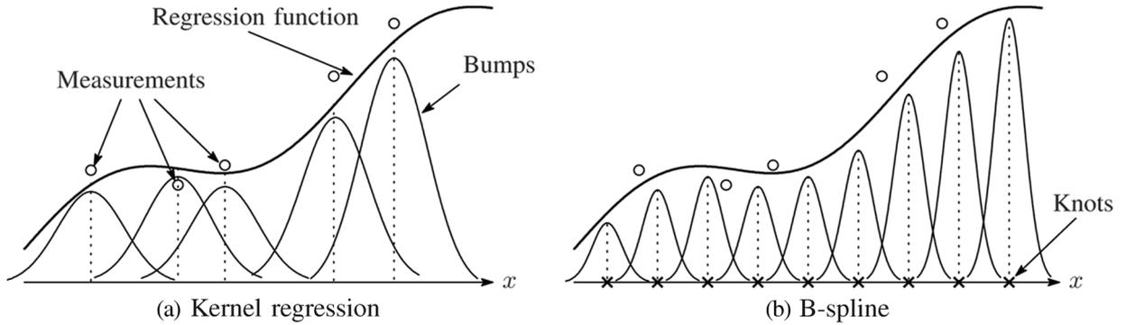
Fig. 4. Comparison of the position of knots in (a) kernel regression and (b) classical B-spline methods.
