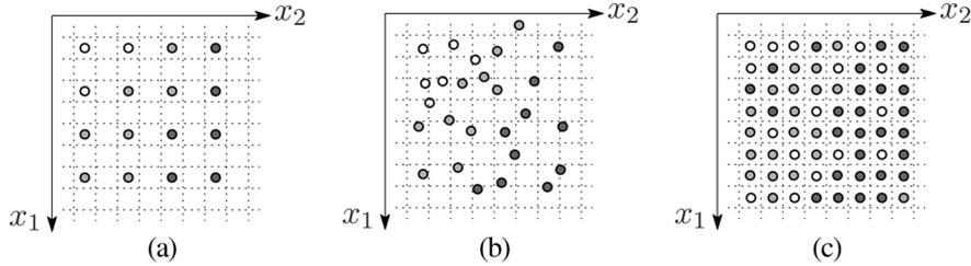
Fig. 1. (a) Interpolation of regularly sampled data. (b) Reconstruction from irregularly sampled data. (c) Denoising.
