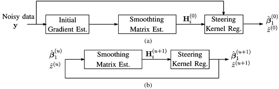
Fig. 10. Block diagram representation of the iterative steering kernel regression. (a) Initialization. (b) Iteration.
