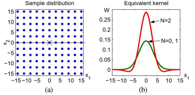
Fig. 5. (a) Uniformly sampled data set. (b) Horizontal slice of the equivalent kernels of orders  $N=0, 1$ , and  $2$  for the regularly sampled data in (a). The kernel  $K_{\mathbf{H}}$  in (20) is modeled as a Gaussian, with the smoothing matrix  $\mathbf{H} = \text{diag}[10, 10]$ .
