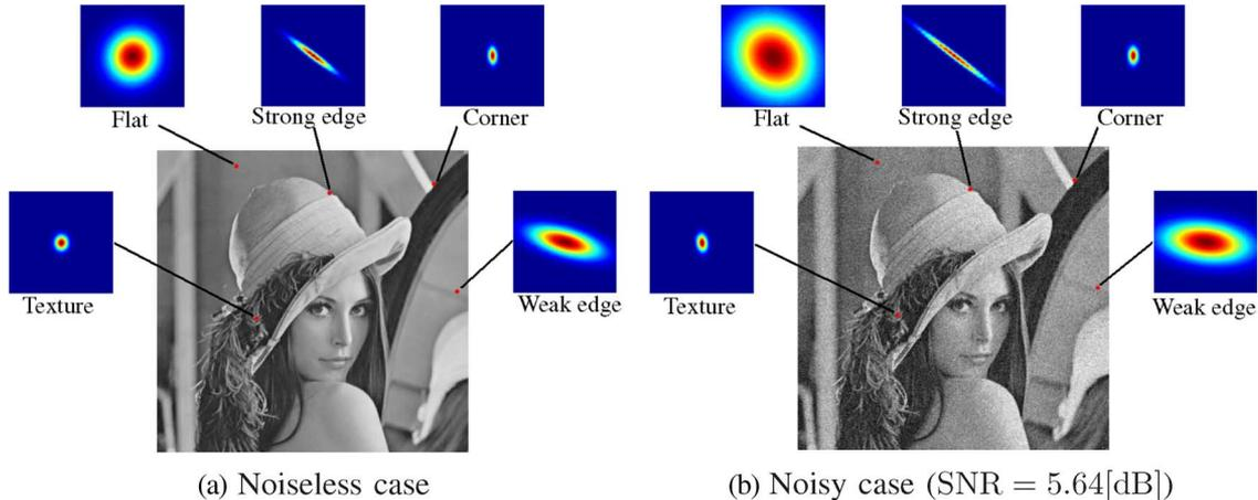
Fig. 11. Footprint examples of steering kernels with covariance matrices  $\{C_i\}$  given by the local orientation estimate (50) at a variety of image structures. (a) The estimated kernel footprints in a noiseless image and (b) the estimated footprints for the same areas of a noisy image (after 7 iterations considering additive Gaussian noise with  $\sigma = 25$  similar to the first experiment of Section IV).
