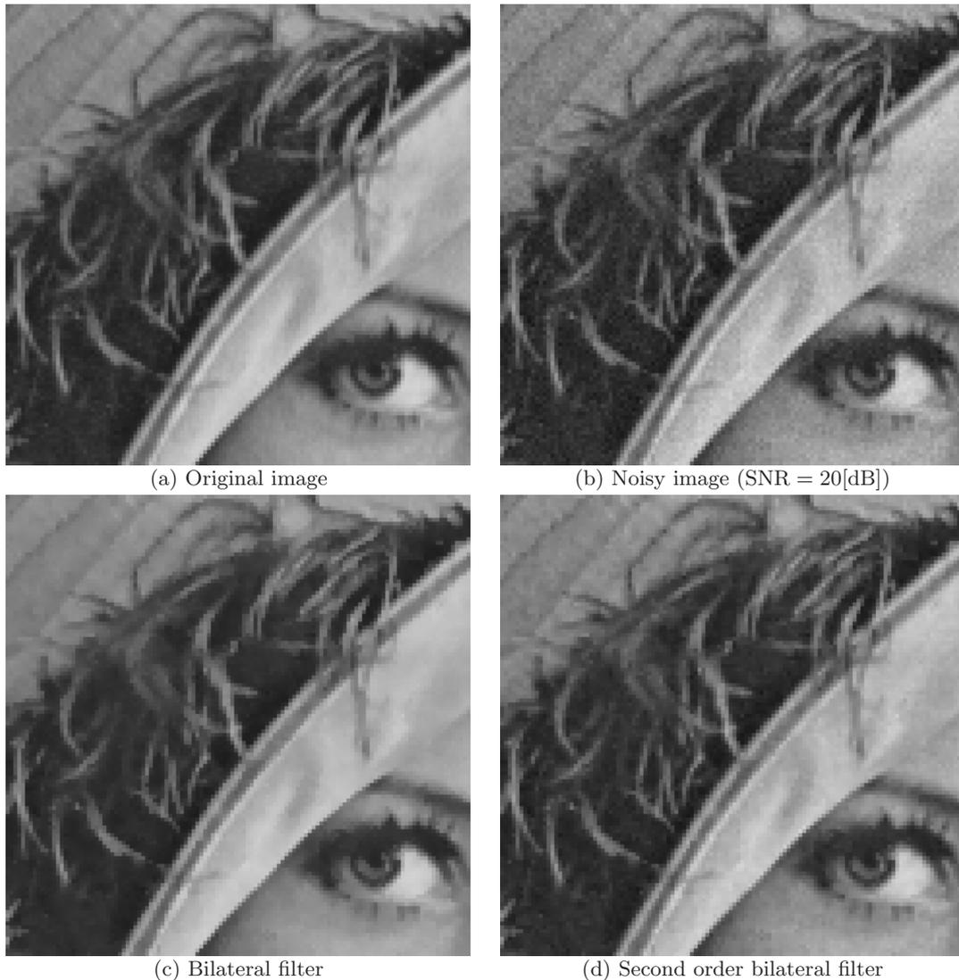
**Figure 4.** Denoising example of higher order bilateral filter (single application) in  $\text{SNR} = 20[\text{dB}]$ : (a) original image, (b) noisy image ( $\text{SNR} = 20[\text{dB}]$ ), and (c)-(d) denoised images by the standard bilateral filter and the second order bilateral filter, respectively. The RMSE values for the denoised images are (c) 4.15 and (d) 3.84.
