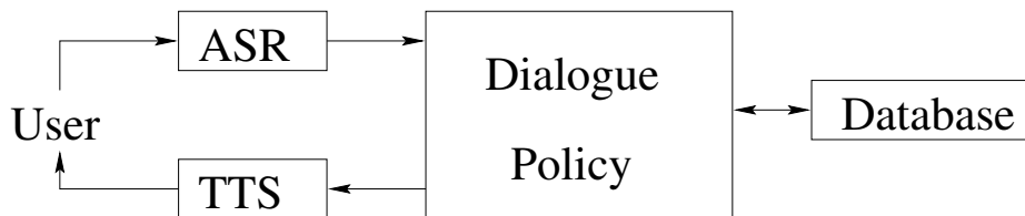
Figure 2: A block diagram representation of a spoken dialogue system. The user gains access to a database by speaking to the system in natural language through the automatic speech recognition system (ASR). The system talks back to the user through a text to speech (TTS) system.
