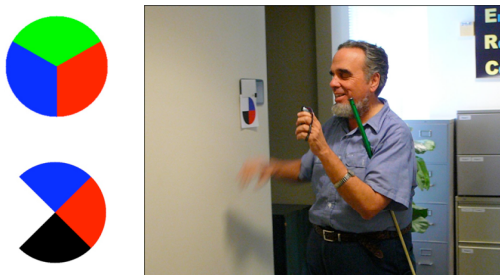
Figure 1. Left: Two versions of our proposed color marker. Right: A blind user operating the cell-phone to detect a marker.
