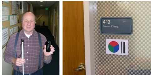
**Fig. 1.** (a) Camera cell phone held by blind user. (b) Color target next to barcode mounted on wall. The distinctive pattern of the color target allows the barcode to be rapidly localized, even against background clutter.
