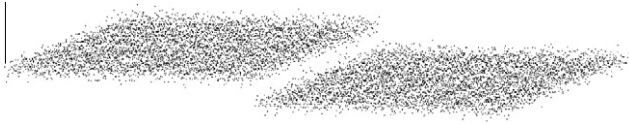
Fig. 2. Synthetically generated data representing a curb with height h equal to 5 units, with added Gaussian noise (in the vertical direction) with standard deviation \sigma equal to 1 unit.
