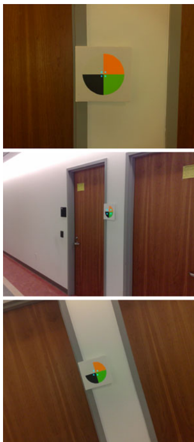
Fig. 1 Our color marker, seen from different viewpoint and with different camera rotations. The blue superimposed crosses represent a fixed-size ‘probe’
