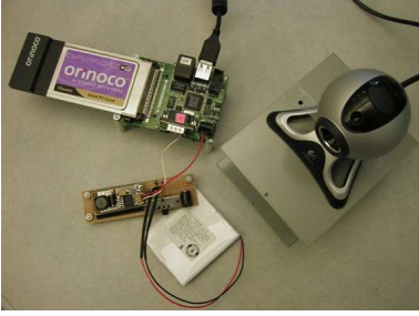
Figure 2. A Meerkats node. Visible are the Crossbow Stargate board with an Orinoco Wi-Fi card and Logitech webcam, the battery (white), and the DC-DC voltage regulator.
