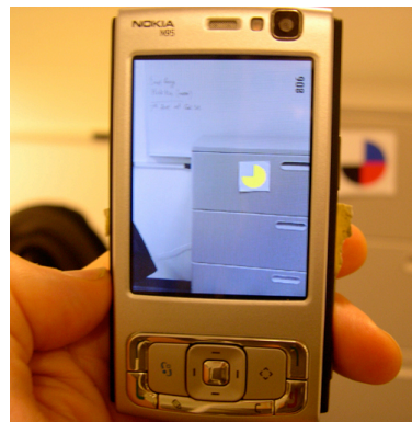
Fig. 1. Marker detection and segmentation (shown in yellow) on the cell phone.
