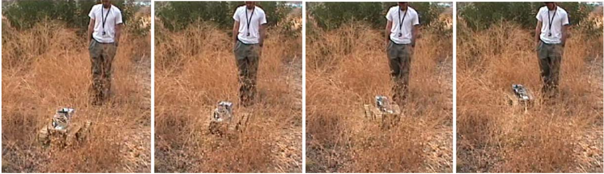
Figure 17. Obstacle avoidance in tall grass using laser-based foliage classification.
