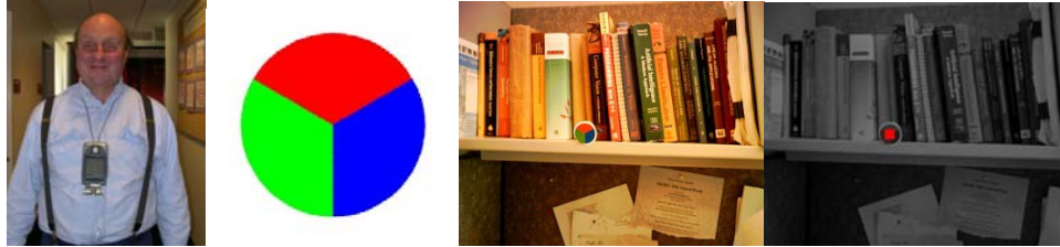
Figure 1: (a) PDA with camera worn by visually impaired user. (b) Colour target consists of three colour patches. (c) Target shown in cluttered environment. (d) Detection result from (c) indicated by red square.
