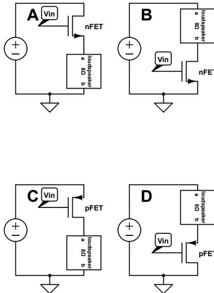
Figure 3: Various ways to arrange an FET and a loudspeaker in series to control the loudspeaker.
