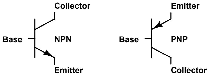
Figure 1: The symbols for bipolar transistors have an arrow marking the direction of conventional current flow (from positive to negative) on the emitter terminal. Current flowing in that direction between the base and emitter cause a larger current ( $\beta$  times as much) in the same direction between collector and emitter. In a phototransistor, the base current results from carriers being excited by photons differently on each side of the junctions.
