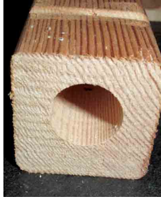
(a) End view of the block showing the finger hole and holes for LED and photodetector.
