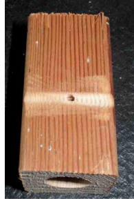
(b) Top view of the block showing the hole for the LED and channels for taking the wires out the side of the block.
