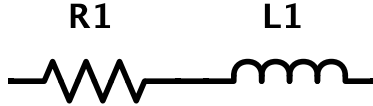
Figure 1: We often model actual inductors as an inductance ( L_1 ) in series with the resistance of the wire used to make the inductor ( R_1 ).
