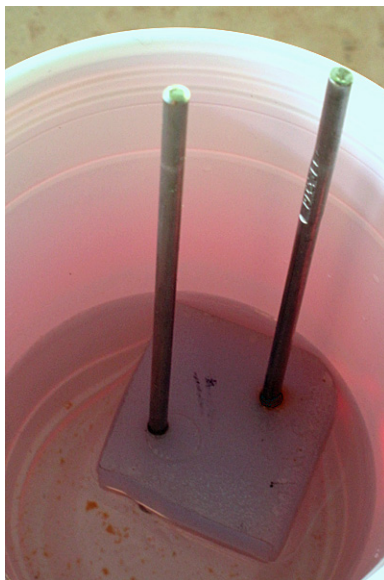
Figure 3: Stainless steel electrodes made from 1/8" 316L stainless steel welding rod.
