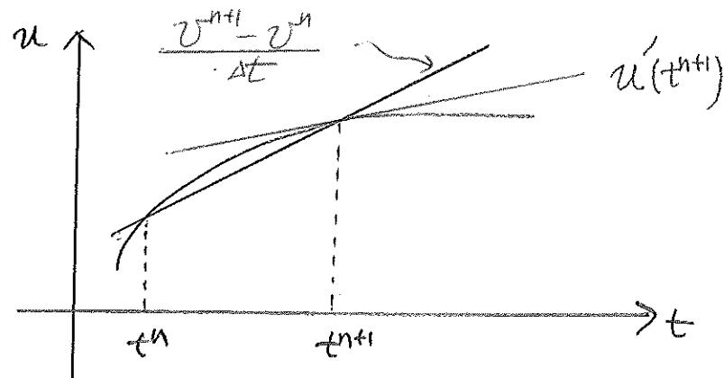
Rmk The backward Euler's method must be solved for  $U^{n+1}$  using an implicit method that often requires iterative numerical solutions for solution convergence for  $U^{n+1}$ .
