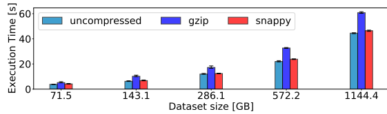
Figure 5: Arrow-Spark leverages compression: Execution time for Arrow-Spark with different compression techniques for parquet data.
