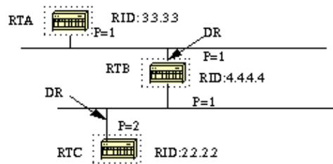
In the above diagram, RTA and RTB have the same interface priority but RTB has a higher RID. RTB would be DR on that segment. RTC has a higher priority than RTB. RTC is DR on that segment.
