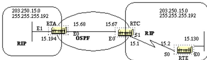
To illustrate, suppose RTA, RTC, and RTE are running RIP. RTC and RTA are also running OSPF. Both RTC and RTA are doing redistribution between RIP and OSPF. Let us assume that you do not want the RIP coming from RTE to be injected into the OSPF domain so you put a passive interface for RIP on E0 of RTC. However, you have allowed the RIP coming from RTA to be injected into OSPF. Here is the outcome:
