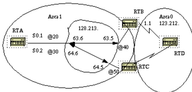
In the above diagram, on RTA, we can split Serial 0 into two point-to-point subinterfaces, S0.1 and S0.2. This way, OSPF will consider the cloud as a set of point-to-point links rather than one multi-access network. The only drawback for the point-to-point is that each segment will belong to a different subnet. This might
