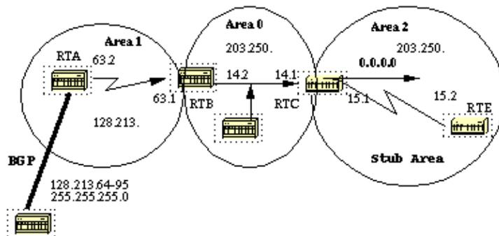
Assume that area 2 is to be configured as a stub area. The following example will show the routing table of RTE before and after configuring area 2 as stub.
