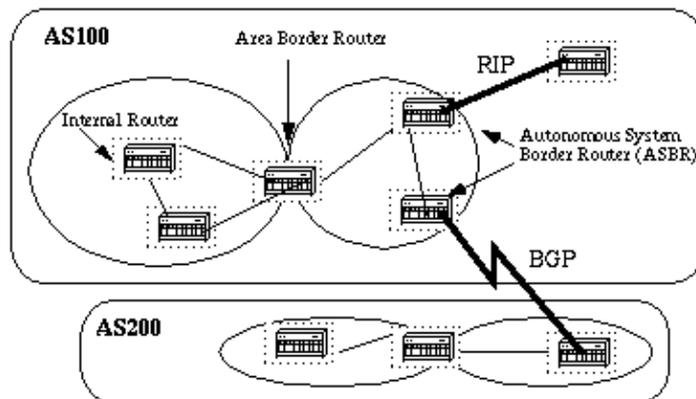
An area is interface specific. A router that has all of its interfaces within the same area is called an internal router (IR). A router that has interfaces in multiple areas is called an area border router (ABR). Routers that act as gateways (redistribution) between OSPF and other routing protocols (IGRP, EIGRP, IS-IS, RIP, BGP, Static) or other instances of the OSPF routing process are called autonomous system boundary router (ASBR). Any router can be an ABR or an ASBR.
