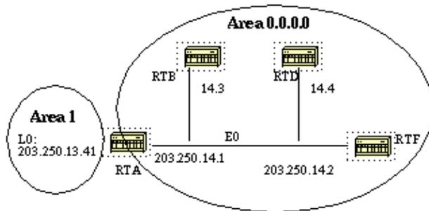
RTA, RTB, RTD, and RTF share a common segment (E0) in area 0.0.0.0. The following are the configs of RTA and RTF. RTB and RTD should have a similar configuration to RTF and will not be included.
