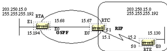
Assume that RTE is injecting a default-route 0.0.0.0 into RIP. RTC will have a gateway of last resort of 203.250.15.2. RTC will not propagate the default to RTA until we configure RTC with a **default-information originate** command.
