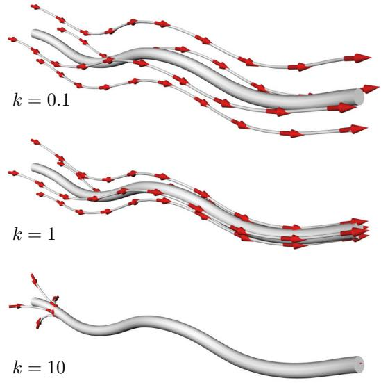
Fig. 5. A feature line (thick) with surrounding streamlines of  $\mathbf{h}$ . The larger the value of  $k$ , the stronger is the attracting behavior of  $\mathbf{h}$ .
