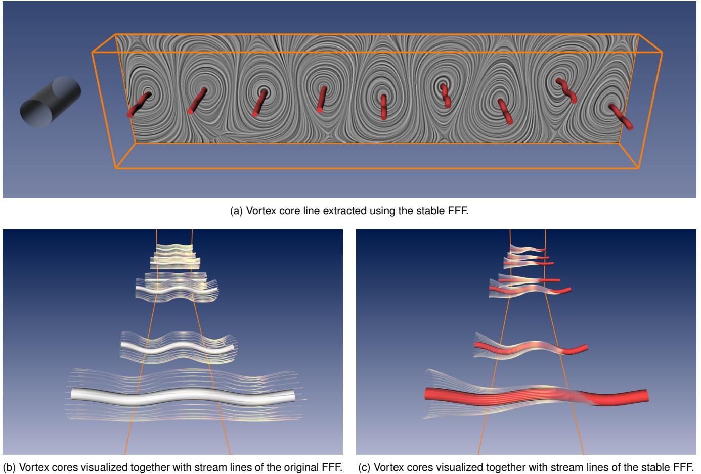
(b) Vortex cores visualized together with stream lines of the original FFF.
