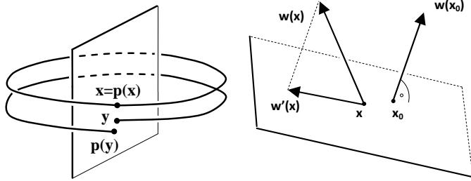
(a) Poincaré map  $p$  with the fix point  $x = p(x)$  corresponding to the closed stream line.  $p$  describes a discrete dynamical system on the plane which can have attracting, repelling, or saddle behavior.
