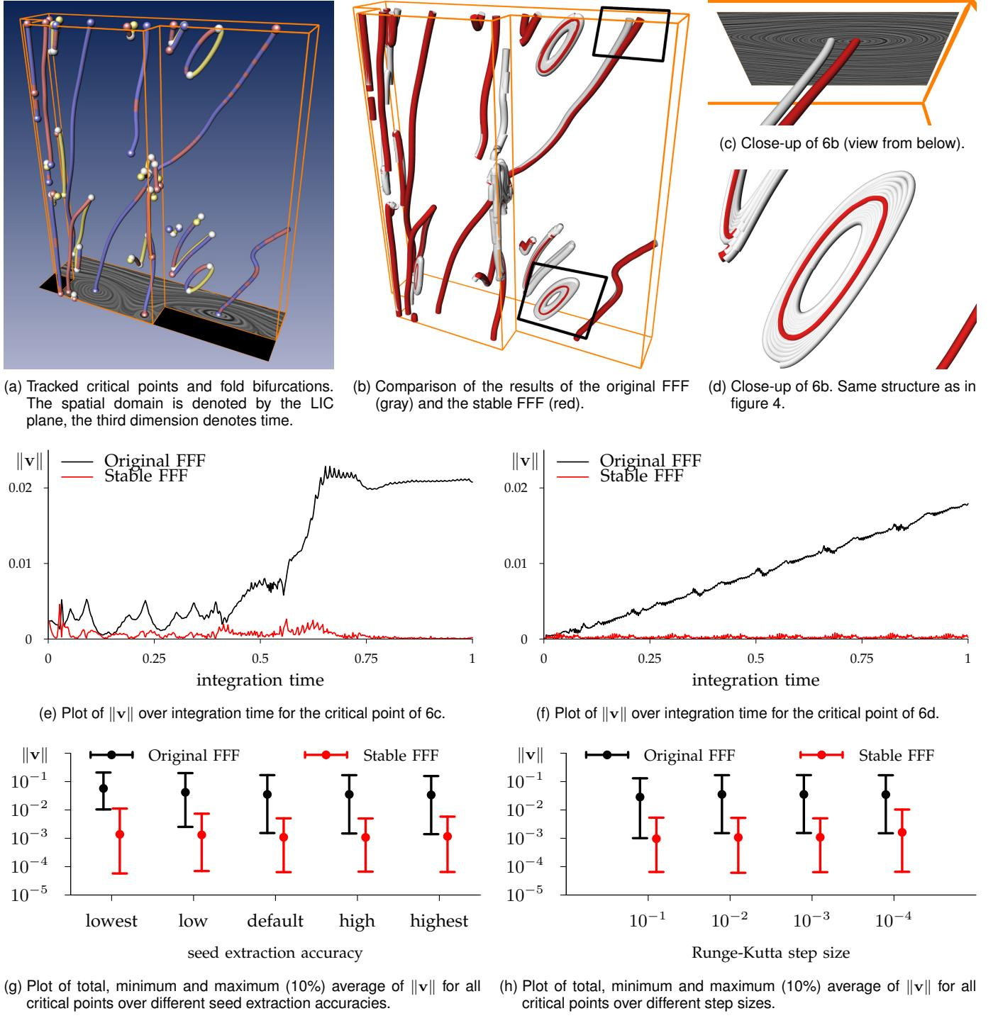
Fig. 6. Cavity data set. Topological visualizations and statistical analysis of the results of the original and the stable FFF approaches. The results have been obtained using an adaptive Runge-Kutta scheme of 4th order except for 6h.
