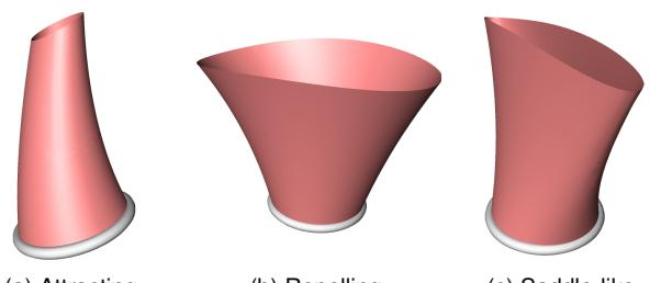
Fig. 3. Local behavior of stream lines around a non-critical point  $x_0$  (images from [23]).
