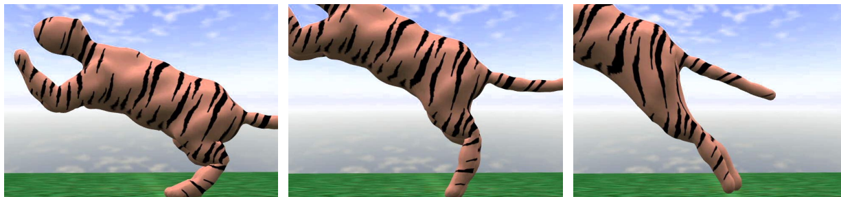
Figure 6: An application of an elastic triangulated mesh. The “tiger” skin is modeled as a spring mesh with stiffness coefficients calculated as described in the paper. As the underlying skeleton moves, the muscles deform, and the skin should move smoothly with the nearby muscle to create a realistic motion.
