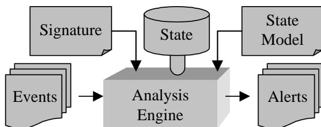
Figure 2. Analysis Engine Architecture.
