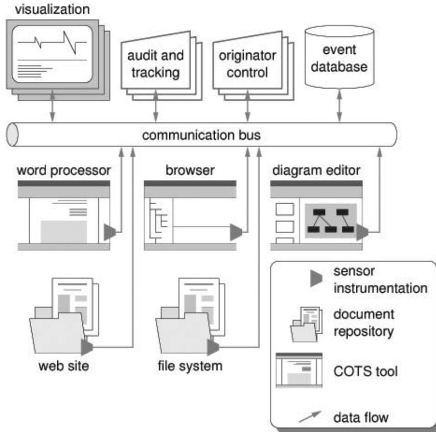
Figure 1. Document Tracking and Control System Architecture
