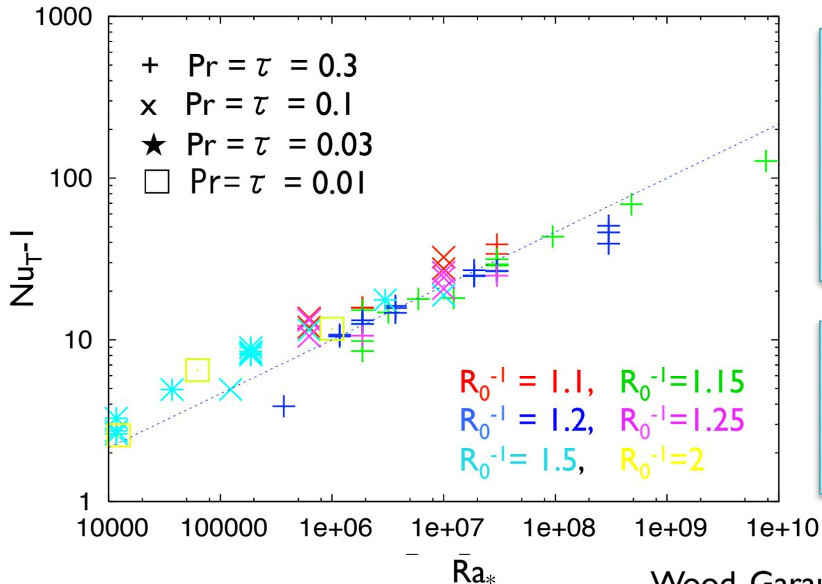
Scaling as in Rayleigh-Benard convection for wall-bounded flows but with turbulent boundary layer
