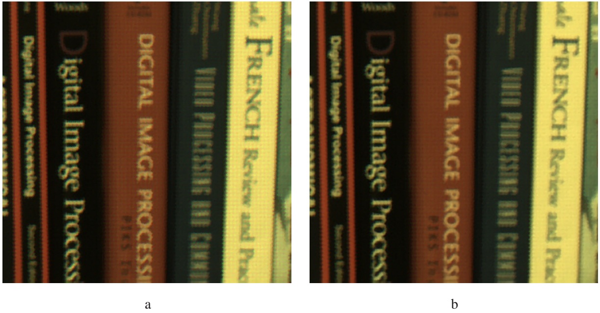
Fig. 14. Multi-frame color super-resolution implemented on a real data sequence. The result of applying our method on the original un-demosaiced raw LR images (without using the inter color dependence term) is shown in (a). (b) is the result of applying our method on the original un-demosaiced raw LR images.
