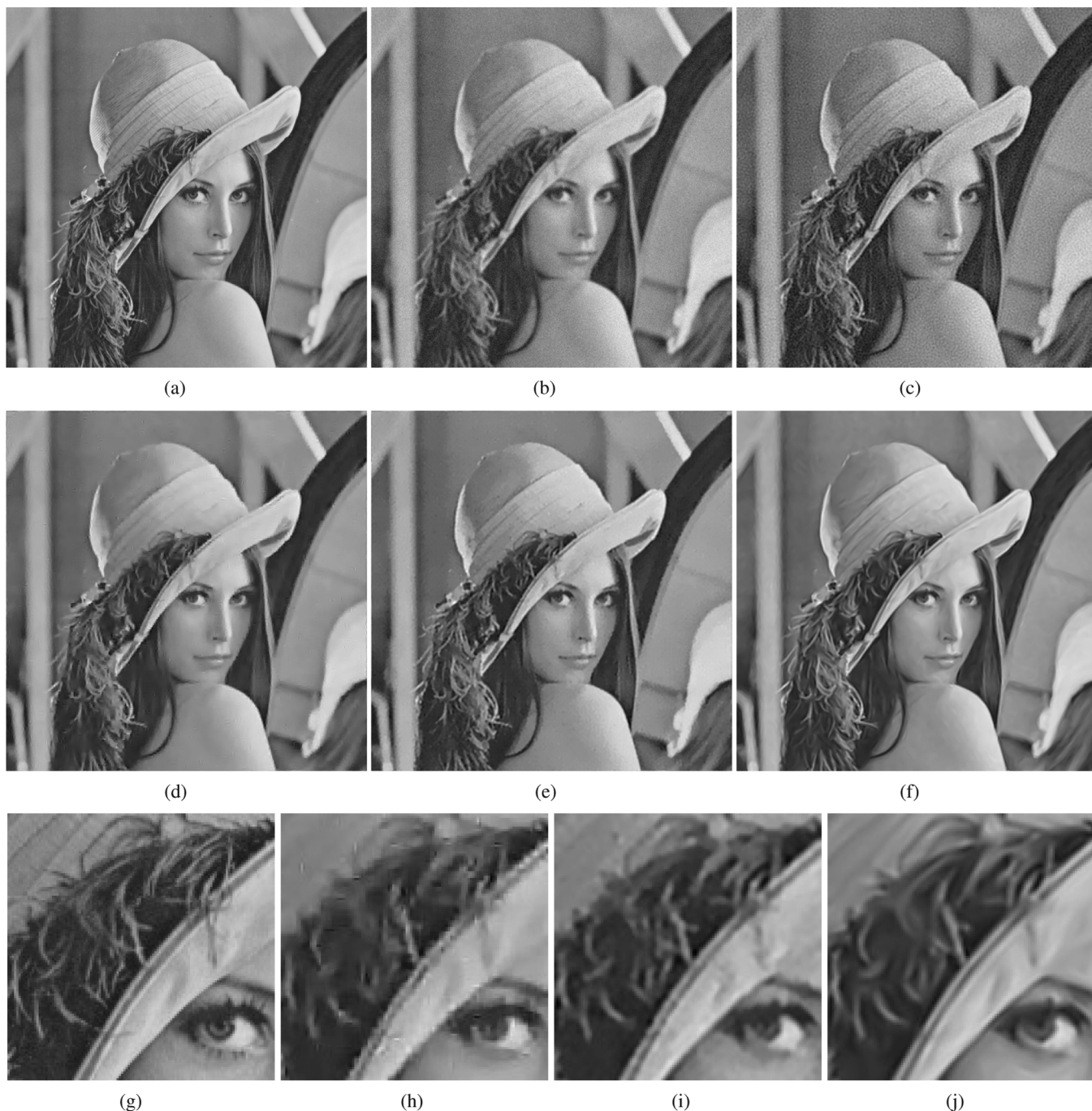
Fig. 12. Single-frame deblurring simulation of the Lena image: (a) original Lena image, (b) degraded image by blurring with a 5 \times 5 Gaussian PSF ( \text{STD} = 1.5 ) and adding white Gaussian noise ( \text{BSNR} = 15 [dB]), (c) restored image by the Wiener filter method with smoothing parameter of 0.05 [13], (d) restored image by ForWaRD [25], (e) restored image by LPA-ICI [11], and (f) restored image by AKTV ((26) with q = 2 , q_r = 1 , N = 1 , and steering kernels (33)). The corresponding RMSE values for (b)–(f) are 10.78, 11.18, 7.55, 6.76, and 6.12, respectively. A selected sections of (a) and (d)–(f) are zoomed in (g)–(j), respectively.
