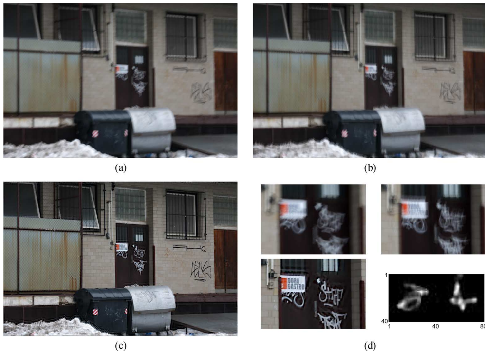
Fig. 14. Real data set. (a) and (b) Two input blurry images of size 2048 \times 1536 . (c) Estimated output sharp image using the proposed algorithm. (d) Closeups of the input images and the output and estimated PSFs of size 40 \times 40 .
