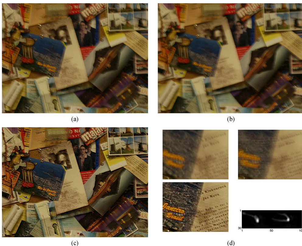
Fig. 13. Real data set. (a) and (b) Two input blurry images of size 2048 \times 1536 . (c) Estimated output sharp image using the proposed algorithm. (d) Closeups of the input images and the output, and estimated PSFs of size 50 \times 30 .
