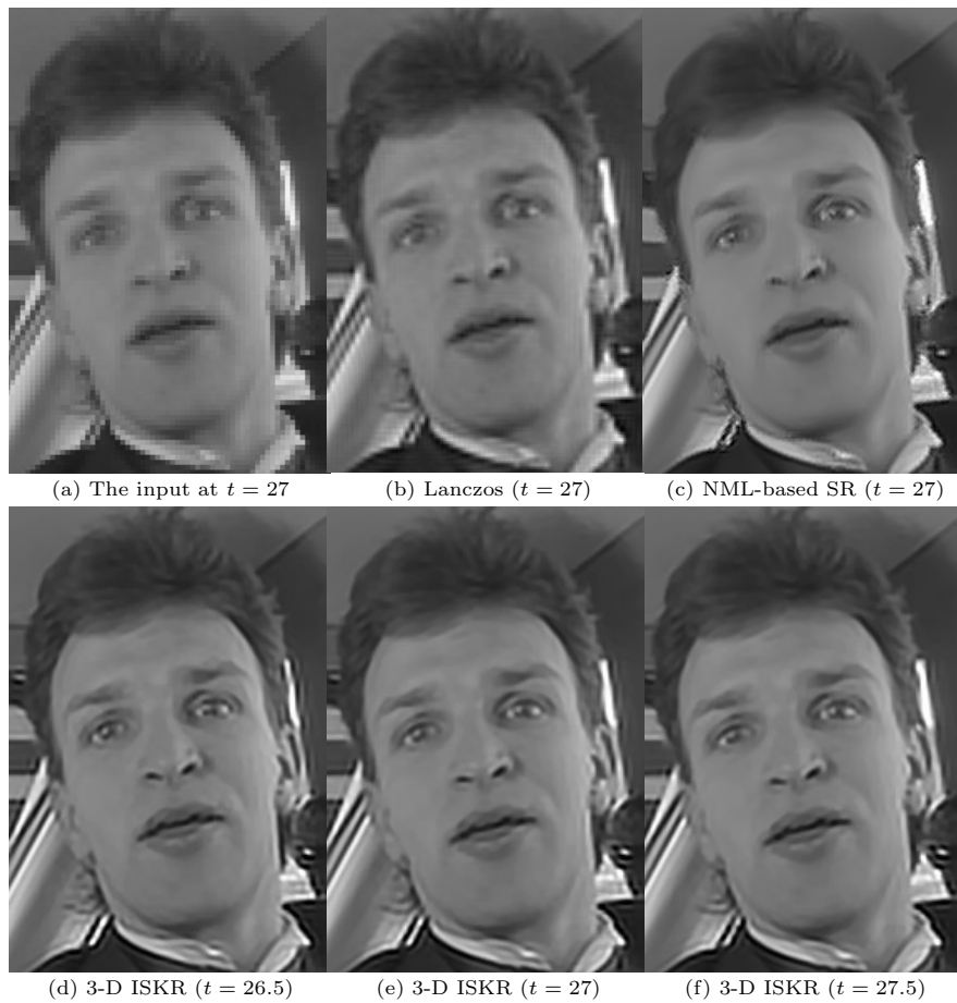
FIGURE 3.14: A Carphone example of video upscaling with spatial upscaling factor 1 : 2: (a) the input video frame at time t = 27 ( 144 \times 176 , 30 frames), (b)-(c) upscaled frames by Lanczos interpolation and NLM-based SR method [28], respectively, and (d)-(f) upscaled frames by 3-D ISKR at t = 26.5 , 27, and 27.5, respectively.
