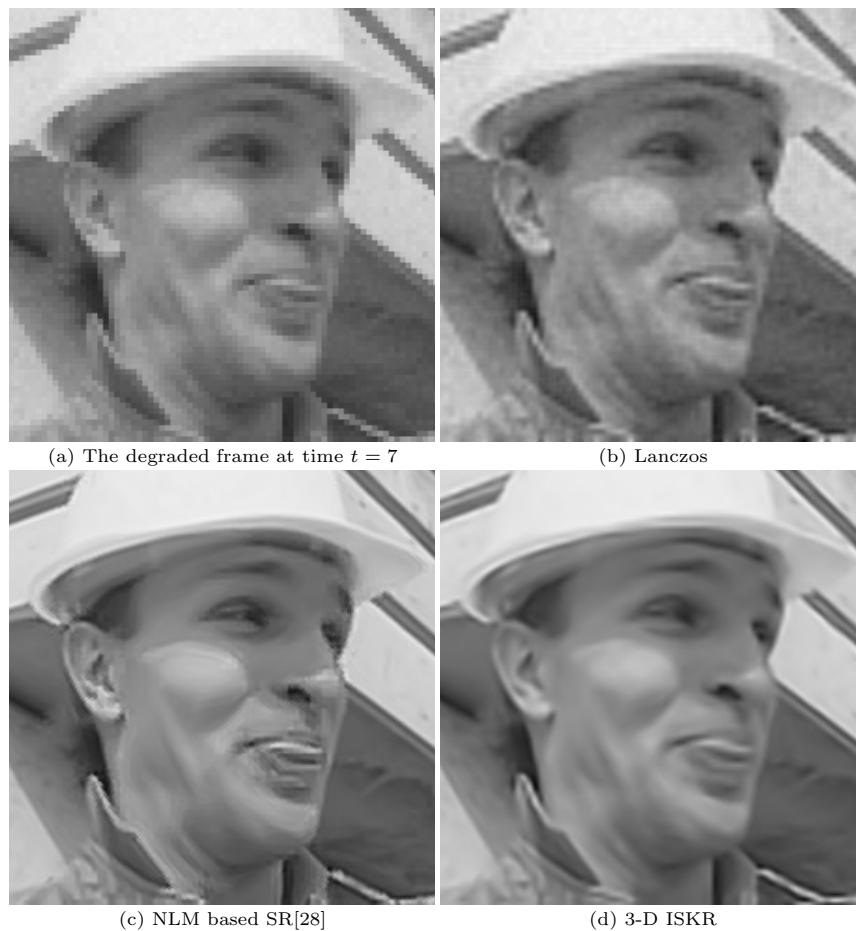
FIGURE 3.11: A video upscaling example using Foreman sequence: (a) the degraded frame at time t = 7 , (b) the upscaled frame by Lanczos interpolation (PSNR = 30.98[dB]), (c) the upscaled frame by NL-means based SR [28] (PSNR = 32.21[dB]), and (d) the upscaled frame by 3-D ISKR (PSNR = 33.58[dB]). Also the PSNR values for all the frames are shown in Figure 3.12(b)
