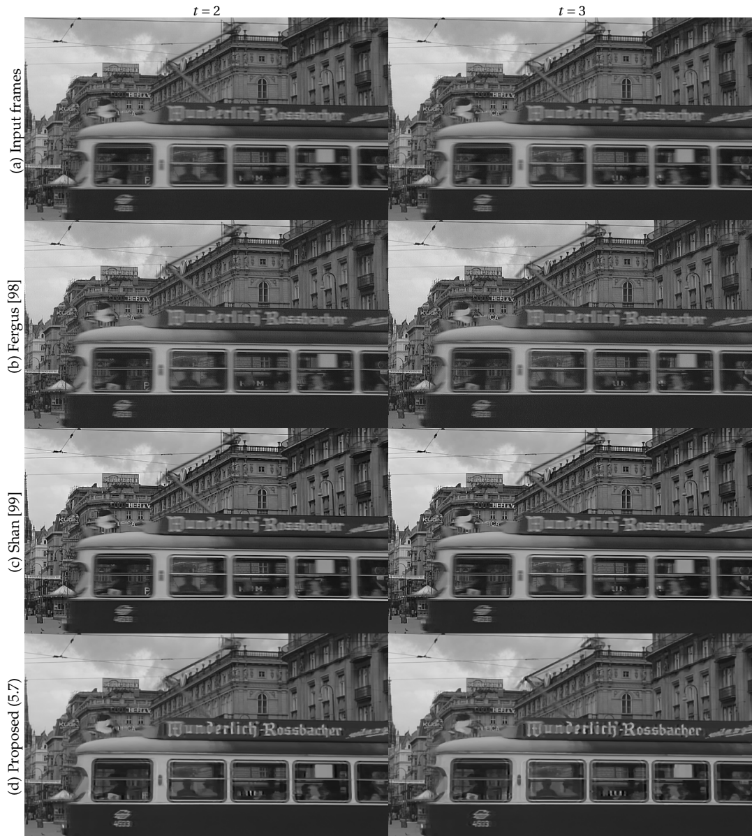
Figure 5.8: A motion (temporal) deblurring example of the StreetCar sequence ( 120 \times 290 , 5 frames) with real motion blur: (a) 2 frames of the ground truth at times t = 2 to 3, (b)-(c) the deblurred frames by Fergus’s method [98], Shan’s method [99], and (d) the deblurred frames by the proposed 3-D TV method (5.7) using a 1 \times 1 \times 8 uniform PSF.
