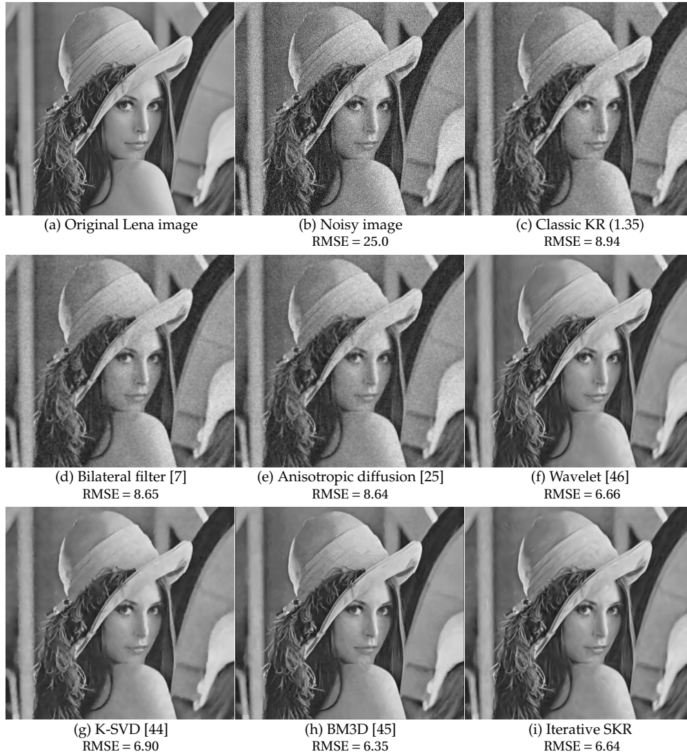
Figure 2.14: An example of Gaussian noise removal with the Lena image: (a) the original Lena image, (b) the noise-ridden image that we generated by adding white Gaussian noise with standard deviation 25 (SNR = 5.64[dB]), (c) the second order classic KR (1.35), (d) bilateral filter [7], (e) anisotropic diffusion [25], (f) a wavelet method [46], (g) K-SVD [44], and (i) Iterative SKR. The corresponding RMSE values are (b)25, (c)8.94, (d)8.65, (e)8.64, (f)6.66, (g)6.90, (h)6.35, and (i) 6.64.
