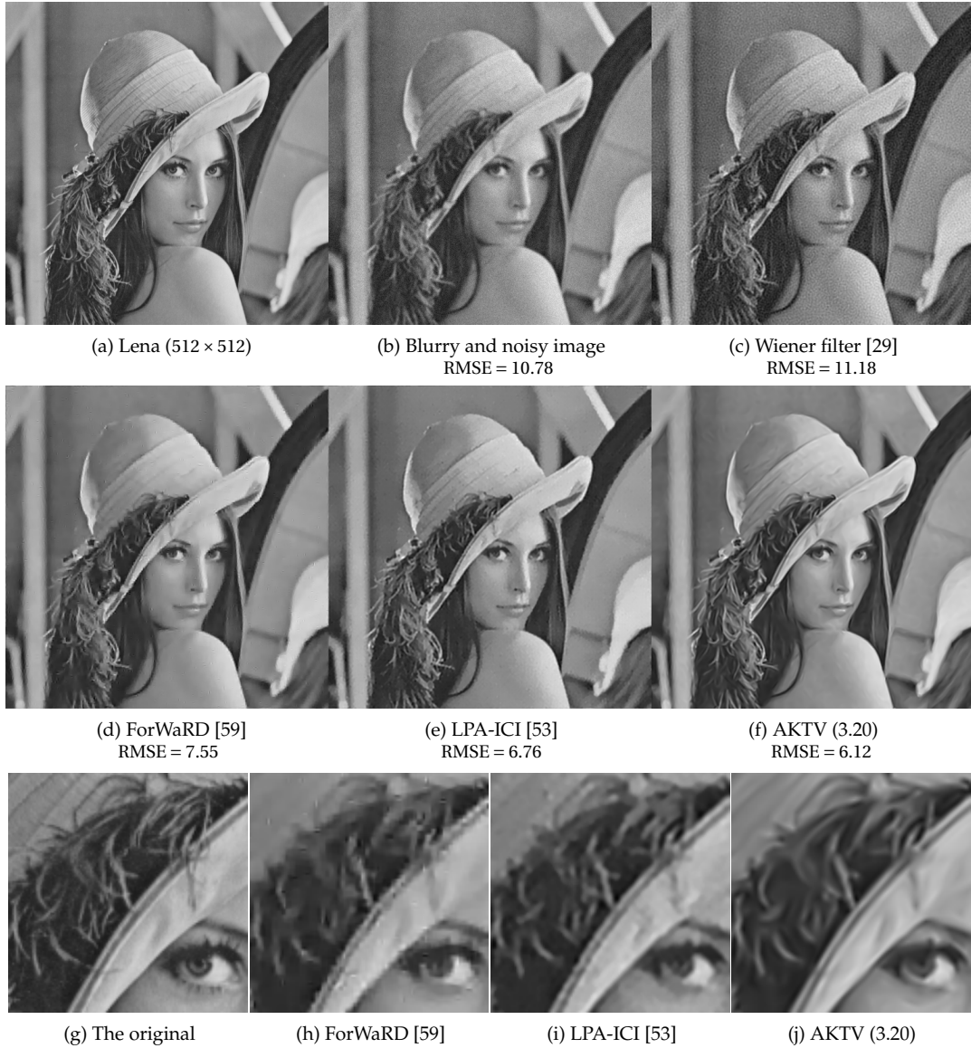
Figure 3.7: Single-frame deblurring simulation of the Lena image: (a) original Lena image, (b) degraded image by blurring with a 5 \times 5 Gaussian PSF (STD = 1.5) and adding white Gaussian noise (BSNR = 15[dB]), (c) restored image by the Wiener filter method with smoothing parameter of 0.05 [29], (d) restored image by ForWaRD [59], (e) restored image by LPA-ICI [53], and (f) restored image by AKTV ((3.20) with q = 1 , N = 1 , and steering kernels (2.9)). The corresponding RMSE values for (b)-(f) are 10.78, 11.18, 7.55, 6.76, and 6.12, respectively. A selected sections of (a) and (d)-(f) are zoomed in (g)-(j), respectively.
