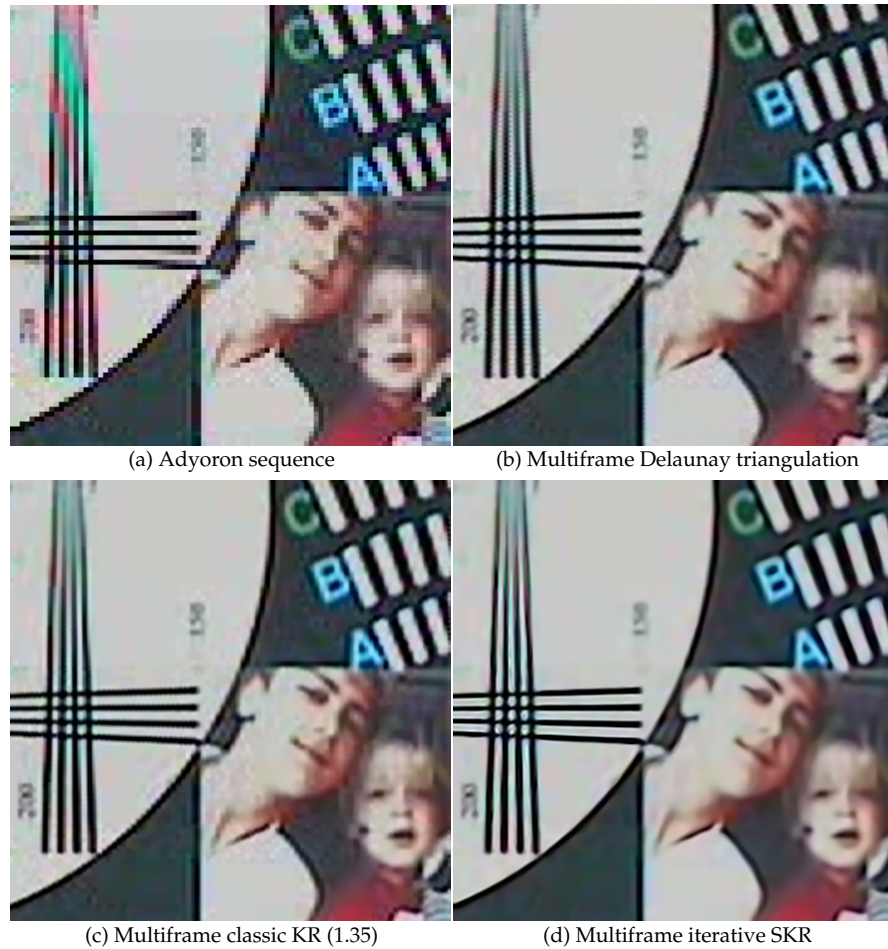
Figure 2.21: An example of resolution enhancement with the Adyoron video sequence: (a) the first video frame of the Adyoron sequence, (b) multiframe Delaunay triangulation, (c) multiframe classic KR (1.35), and (d) multiframe iterative SKR.
