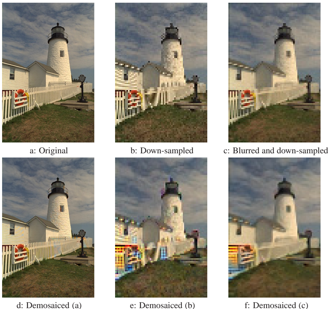
Figure 3.1: A high-resolution image (a) captured by a 3-CCD camera is down-sampled by a factor of four (b). In (c) the image in (a) is blurred by a Gaussian kernel before down-sampling by a factor of 4. The images in (a), (b), and (c) are color-filtered and then demosaiced by the method of [2]. The results are shown in (d), (e), (f), respectively.
