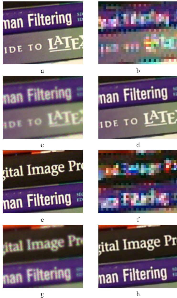
Figure 4.6: A sequence of 250 low-resolution color filtered images where recursively fused (Section 4.2), increasing their resolution by the factor of 4 in each direction. They were further deblurred and demosaiced (Section 4.4), resulting in images with much higher-quality than the input low-resolution frames. In (a) & (e) we see the ground-truth for frames #150 and #200 of size [100 \times 128 \times 3] , and (b) & (f) are the corresponding synthesized low-resolution frames of size [25 \times 32 \times 3] . In (c) & (g) we see the recursively fused high-resolution frames and (d) & (h) of size [100 \times 128 \times 3] show the deblurred-demosaiced frames.
