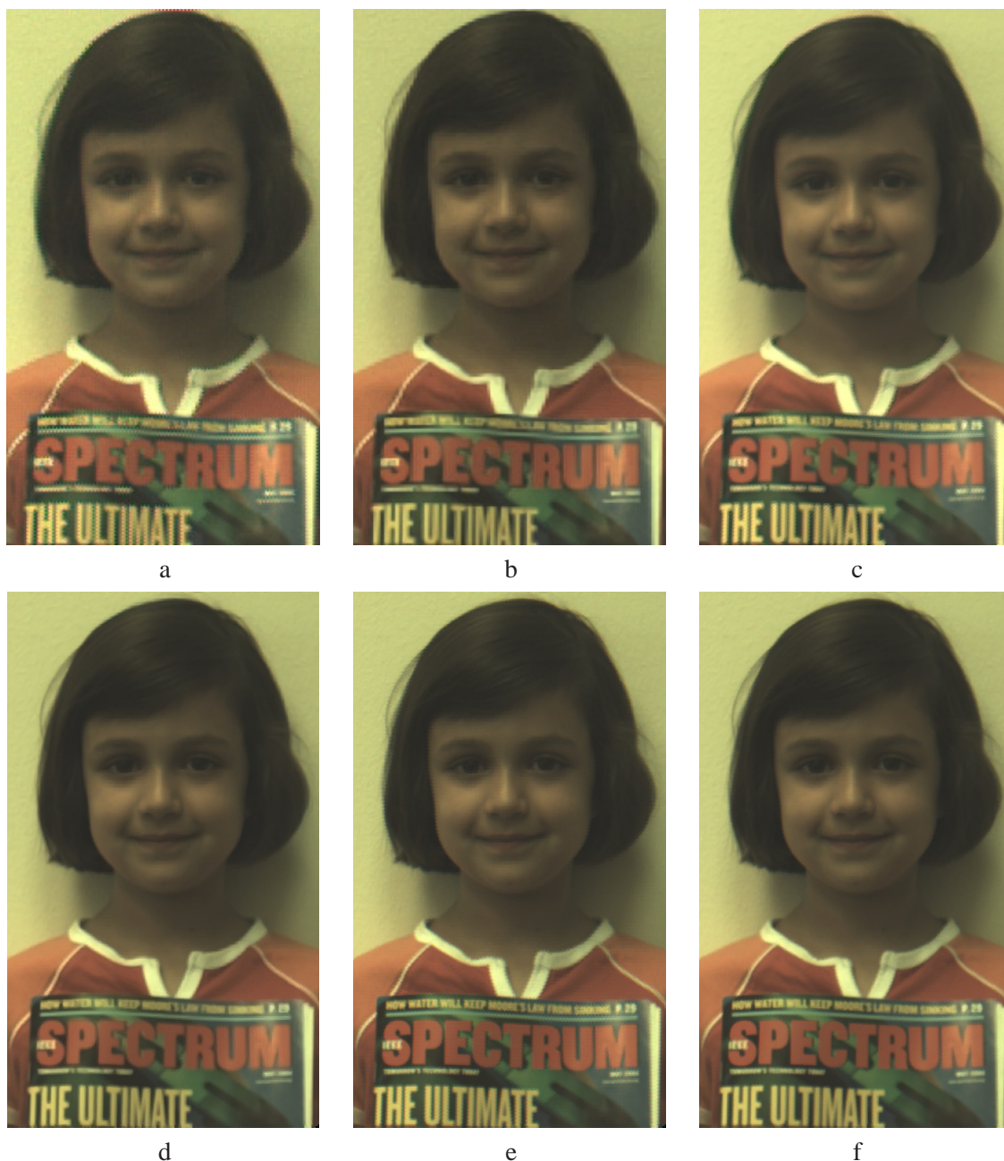
Figure 3.14: Multi-frame color super-resolution implemented on a real data sequence. (a) shows one of the input low-resolution images (of size 290 \times 171 \times 3 ) demosaiced by [3] and (b) is one of the input low-resolution images demosaiced by the more sophisticated [2]. (c) is the result of applying the proposed color-super-resolution method on 31 low-resolution images each demosaiced by [3] method (high-resolution image of size 870 \times 513 \times 3 ). (d) is the result of applying the proposed color-super-resolution method on 31 low-resolution images each demosaiced by [2] method. The result of applying our method on the original mosaiced raw low-resolution images (without using the inter color dependence term) is shown in (e). (f) is the result of applying our method on the original mosaiced raw low-resolution images.
