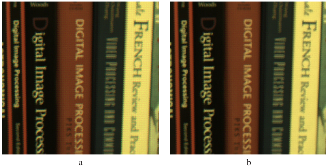
Figure 3.17: Multi-frame color super-resolution implemented on a real data sequence. The result of applying our method on the original mosaiced raw low-resolution images (without using the inter color dependence term) is shown in (a) (high-resolution image of size [423 \times 441 \times 3] ). (b) is the result of applying our method on the original mosaiced raw low-resolution images.
