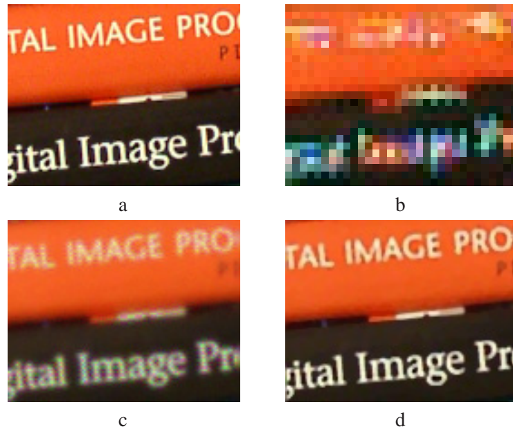
Figure 4.7: A sequence of 250 low-resolution color filtered images where recursively fused (Section 4.2), increasing their resolution by the factor of 4 in each direction. They were further deblurred and demosaiced (Section 4.4), resulting in images with much higher-quality than the input low-resolution frames. In (a) we see the ground-truth for frame #250 of size [100 \times 132 \times 3] , and (b) is the corresponding synthesized low-resolution frame of size [25 \times 32 \times 3] . In (c) we see the recursively fused high-resolution frame and (d) of size [100 \times 128 \times 3] show the deblurred-demosaiced frame.
