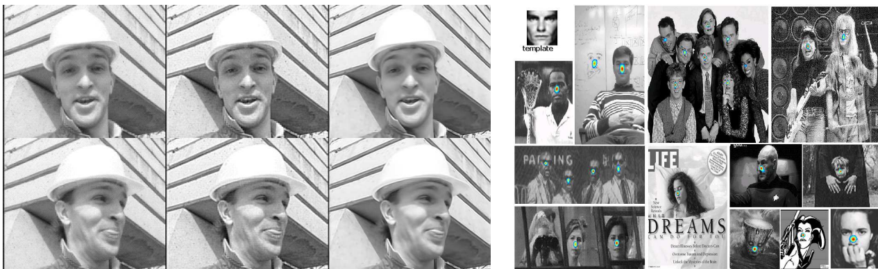
Figure 2: Left: Restoration example. A video upscale example using a real video sequence: Column 1 shows 2 frames from the original video; next column shows the upscaled frames by Lanczos interpolation, and the third column shows the upscaled frames by 3-D SKR. Right: Recognition example. Note that the template example does not actually appear in any of the target images. Colored contours show the center of the detected matching regions.
