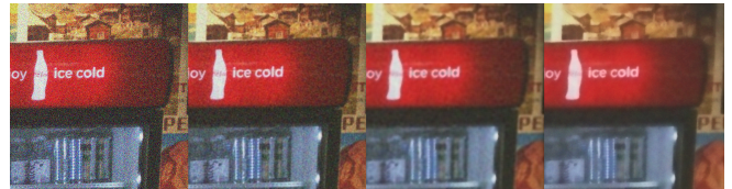
Fig. 7. From left to right, synthetic image with text with additive Gaussian noise with \sigma=85 (SSIM:0.089), 7x7 NLM (SSIM:0.794), 15x15 NLM (SSIM:0.864), pull-push NLM (SSIM:0.874)
