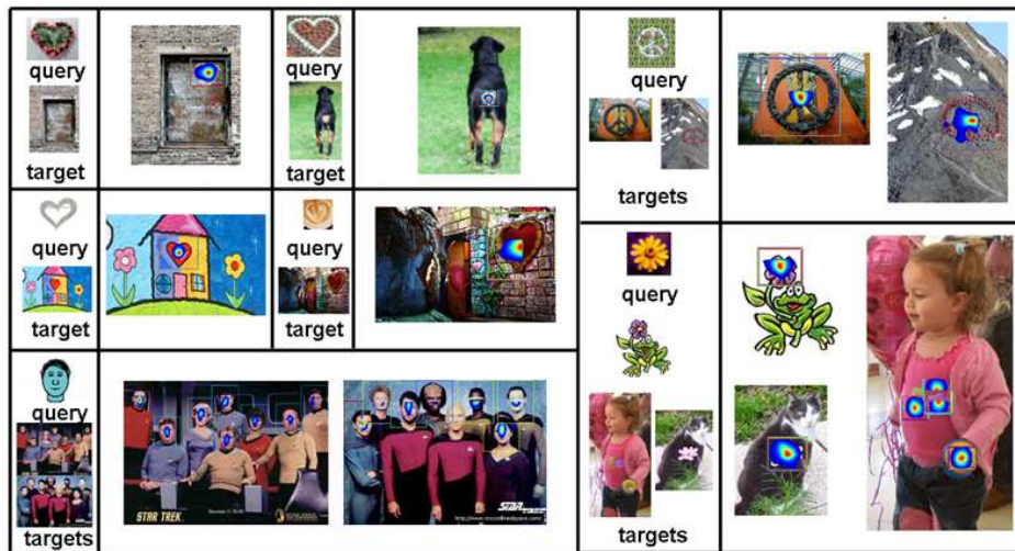
Fig. 7. Query: hearts, hand-drawn face, peace symbol and flower. Some targets and examples of correction detections/ localizations in Shechtman's object test set [5] are shown. Some false positives appeared in a girl's T-shirt and candle. \alpha was set to 0.98.
