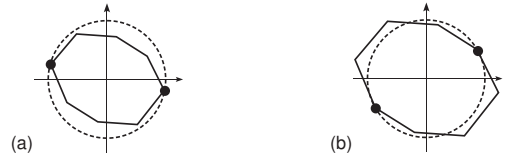
Figure 1: Principal signals and the MAP defining polytope. The dotted circles denote the unit sphere in 2D signal space. The two polygons are different scales of the same MAP defining polytope. (a) A principal signal, obtained at a vertex of the defining polytope. (b) A vertex which does not represent a principal signal.
