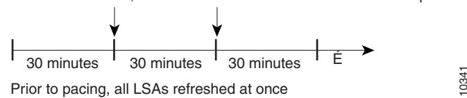
Figure 39 OSPF LSAs on a Single Timer Without Group Pacing
