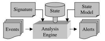
Figure 2. Analysis Engine Architecture.
