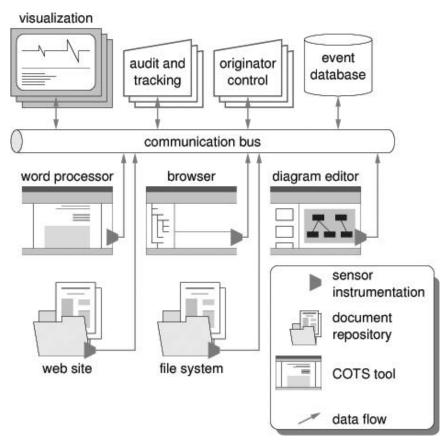
Figue 1. Document Tracking and Control System Architecture
