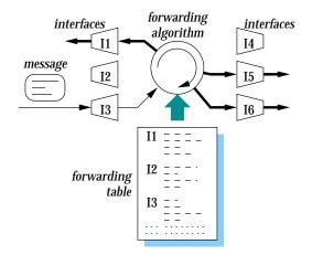
Figure 3: Forwarding in a Content-Based Network's Router
