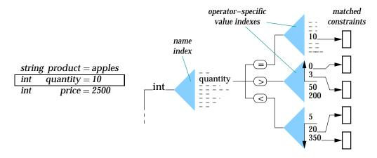
Figure 7: Example of Use of Constraint Index
