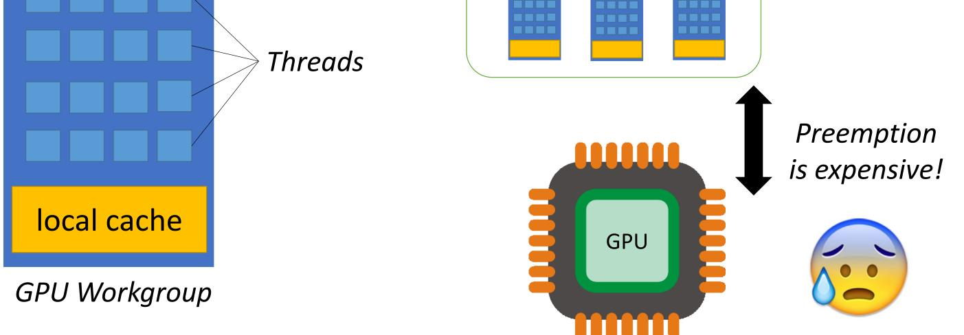
On GPUs, preemption is difficult due to the large state that needs to be saved. A GPU workgroup's state contains up to 256 threads and a local cache. Efficiently saving and restoring is non-trivial.
