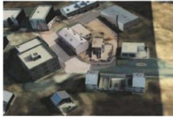
Fig. 18. Video flashlight: video frame is warped and overlaid over model; scene may be visualized from any viewpoint.
