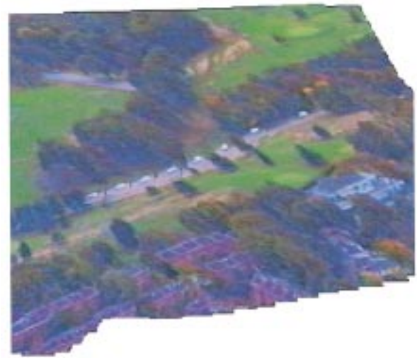
Fig. 25. Synopsis mosaic obtained while tracking a white truck along a road. The appearance of the truck at multiple locations is overlaid on the mosaic.
